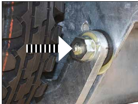
▲ 37/1 Lubrication point on the PRIBOT Hanger assembly tactile shield right/left back the drive wheels
